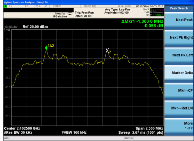
(2Mbps) Channel Separation plot on channel 39-40
