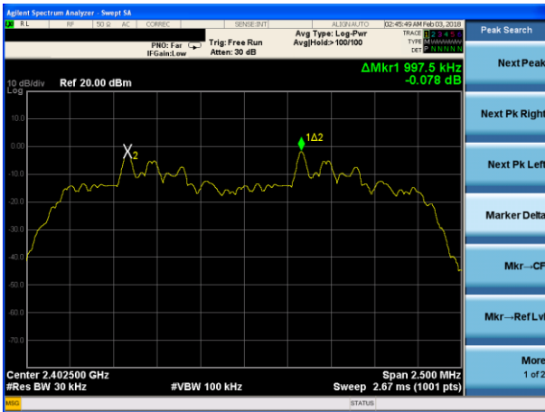
(3Mbps) Channel Separation plot on channel 00-01
