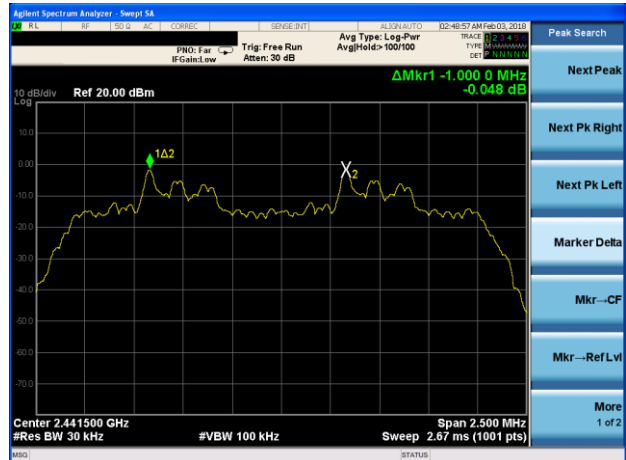
(2Mbps) Channel Separation plot on channel 39-40
