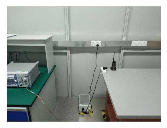
**RADIATED EMISSION TEST SETUP**
