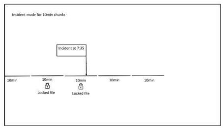
Note on current segment: When Incident Protection Mode is triggered, or if you request a Manual Footage Capture, the current segment will be locked but it will also continue recording until the segment is complete or the device is turned off. For example, if you trigger Incident Protection Mode 3 minutes into a 5 minute segment, your Fly6 will also record the following 2 minutes and add it into the locked file.
