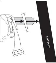
3. While holding the seat post mount against your seat post, wrap the seat post strap around the seat post and pull through the slot at the other end of the Fly6 seat post mount.
