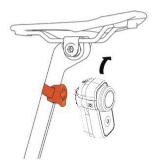
5. You can easily remove your Fly6 from the bike by removing it from the seat post mount with a 1/8th turn **anticlockwise**. You can leave the mount on your bike for next use.
