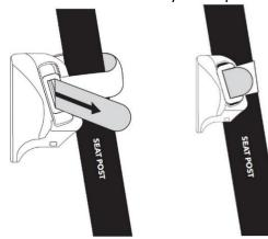
4. To mount your Fly6 align the tabs on the device with the slots in the seat post mount. Turn device **clockwise** a 1/8th turn until you hear a click and then the device will be locked into the seat post mount. Note : The device must be mounted in an upright position as shown.
