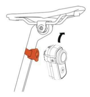
5. You can easily remove your Fly6 from the bike by removing it from the seat post mount with a 1/8th turn **anticlockwise**. You can leave the mount on your bike for next use.
