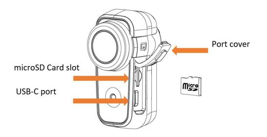
You can insert a microSD card into the microSD card slot of your Fly6 device and press in gently until locked in place. Please ensure the label on the microSD card is facing towards the front of the Fly6, as illustrated above.
