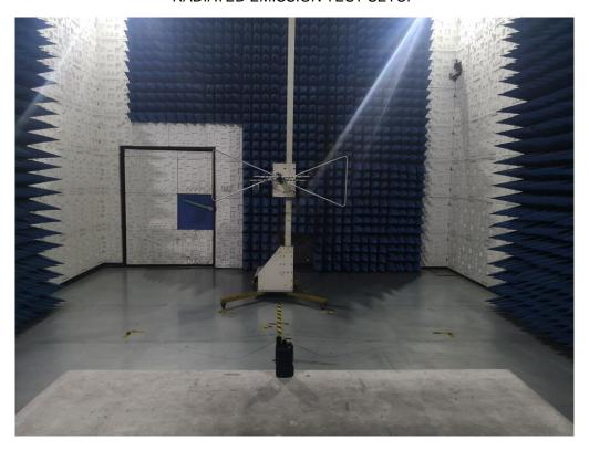
RADIATED EMISSION ABOVE 1G TEST SETUP
