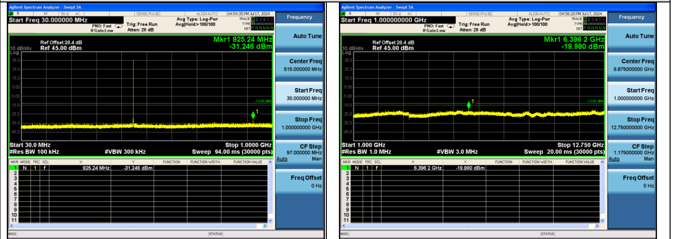
25kHz, FM modulation, Assigned Frequency:462.6500MHz, 4.5W
