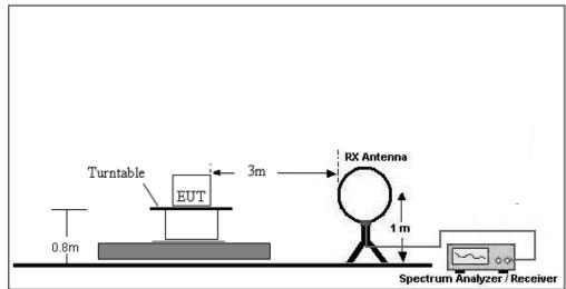
(B) Radiated Emission Test-Up Frequency 30MHz~1GHz
