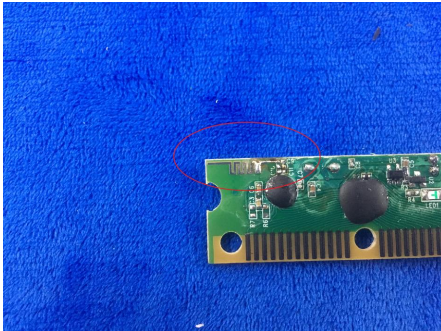
Antenna View (RX)
