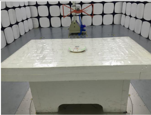
Radiated Spurious Emissions Test Setup Below 1GHz
