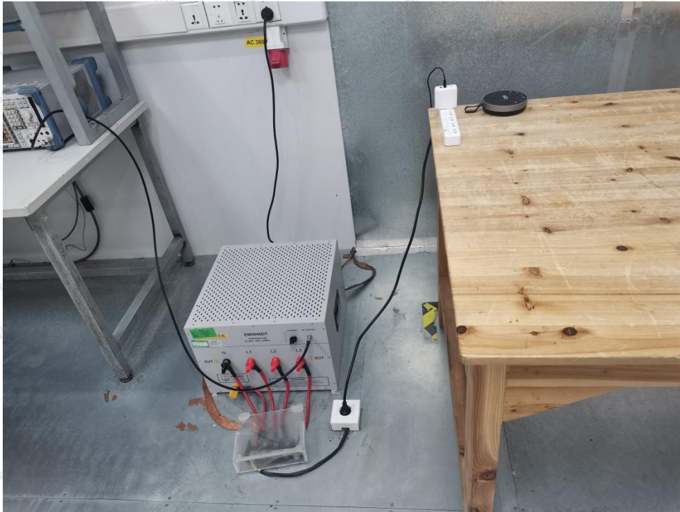
Photo of Conducted Emission Measurement
