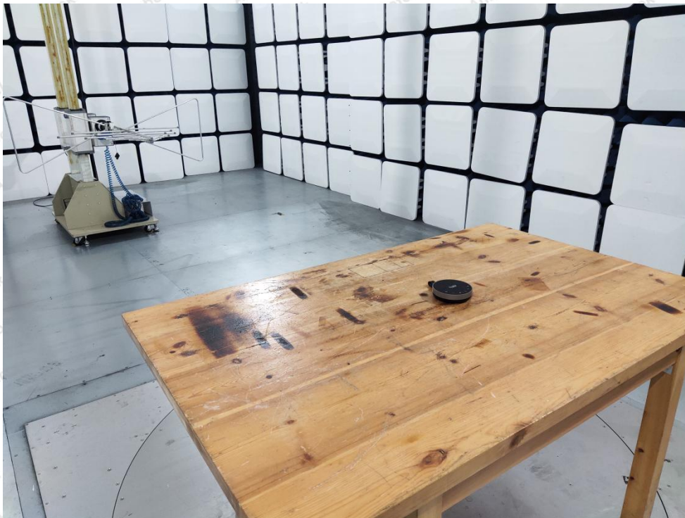
Photo of Radiation Emission Test
