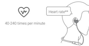
d. If the heart rate isn't within testing range, the device cannot test it, and indicator will flash in red.
