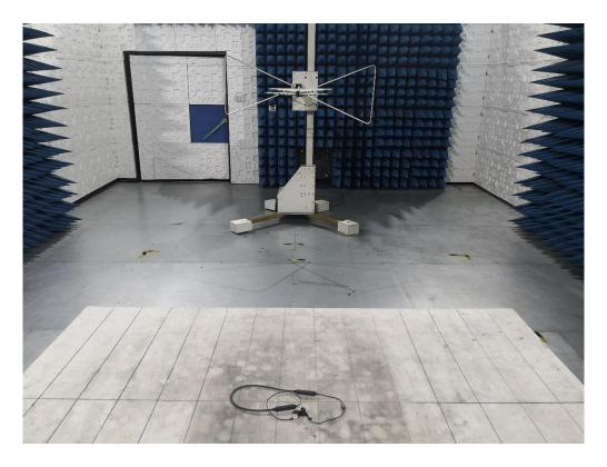
RADIATED EMISSION TEST SETUP ABOVE 1GHZ
