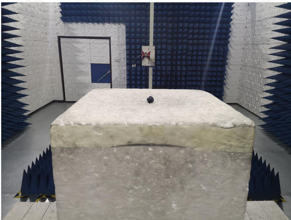
RADIATED EMISSION TEST SETUP ABOVE 1GHZ
