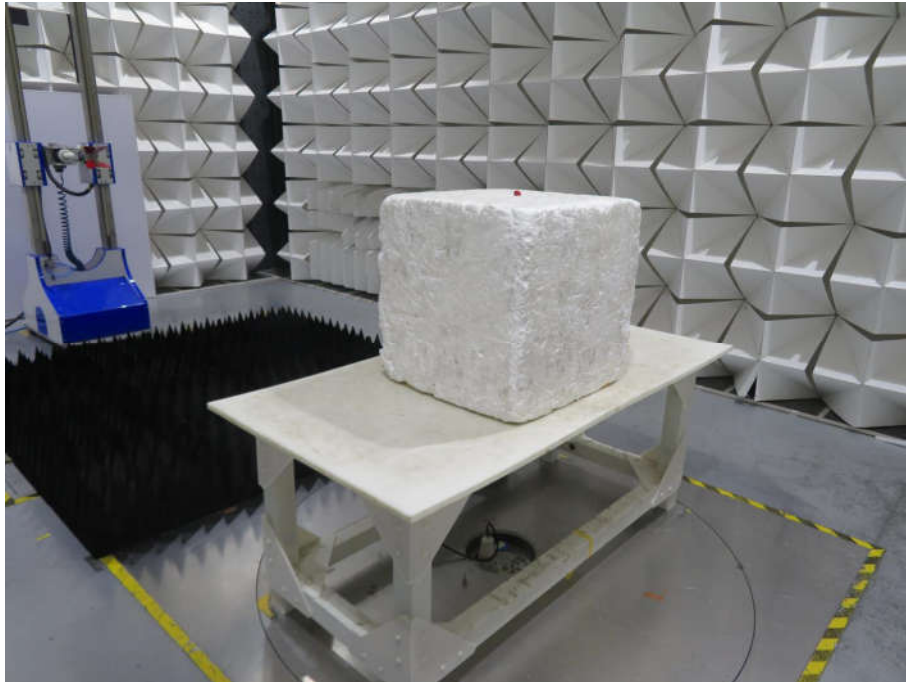
Radiated spurious emission Test Setup-3(Above 1GHz)
