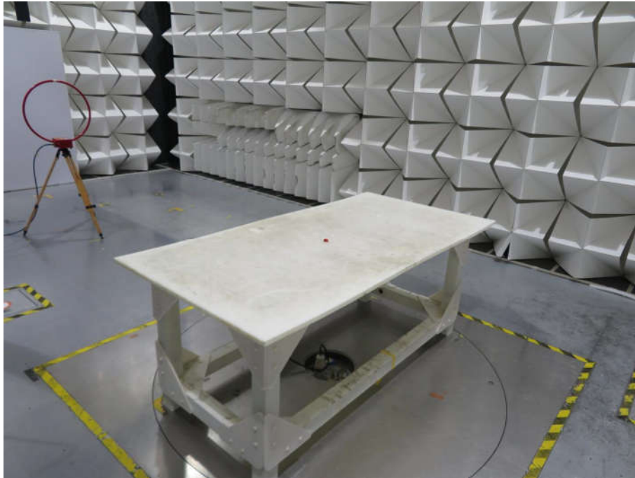
Radiated spurious emission Test Setup-1(Below 30MHz)
