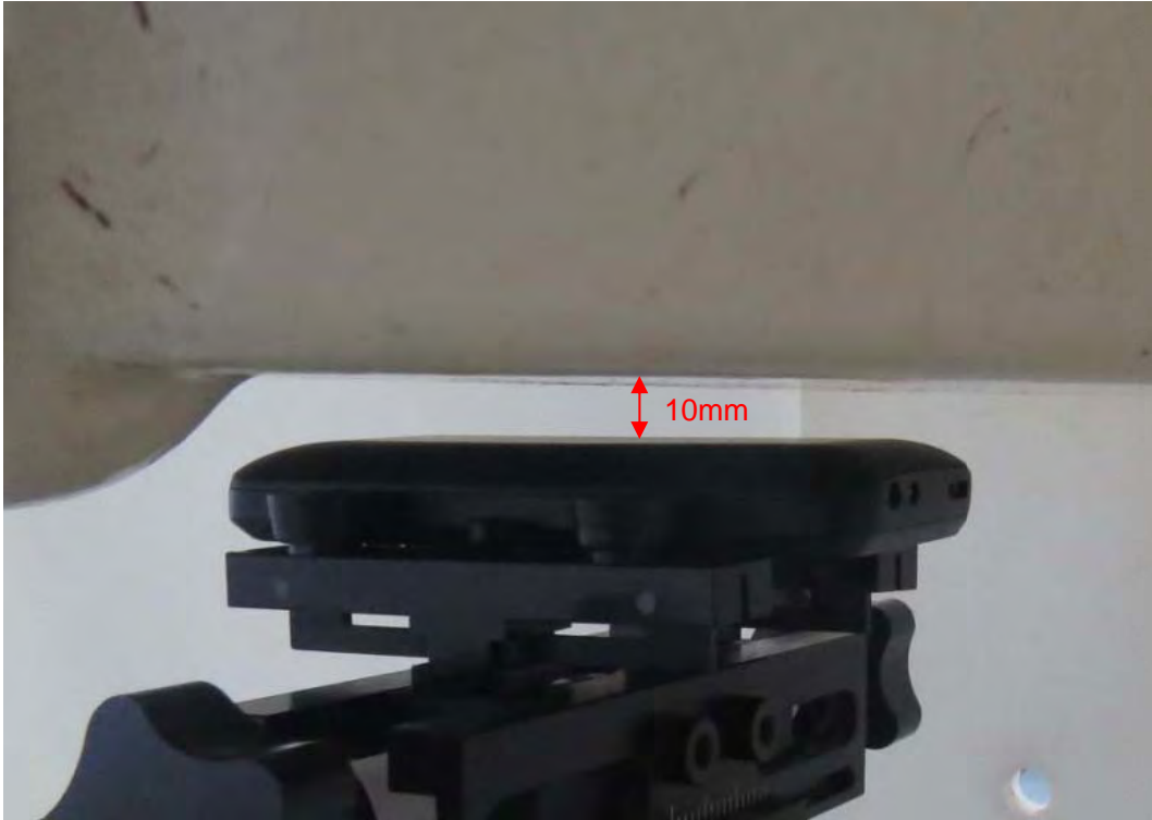
Picture 12: Back Side, the distance from handset to the bottom of the Phantom is 10mm
