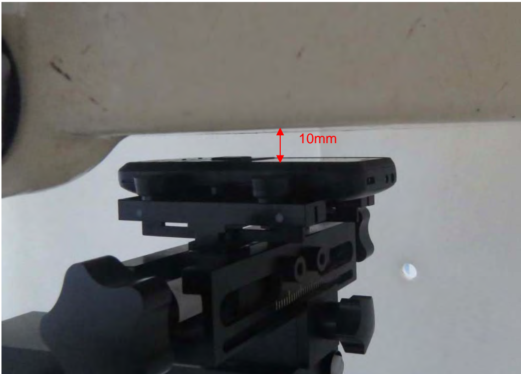
Picture 13: Front Side, the distance from handset to the bottom of the Phantom is 10mm
