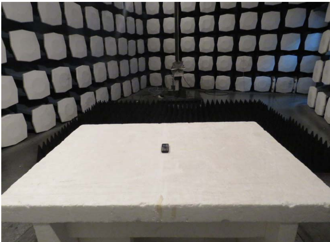
Picture 2: Radiated Spurious Emissions Test setup
