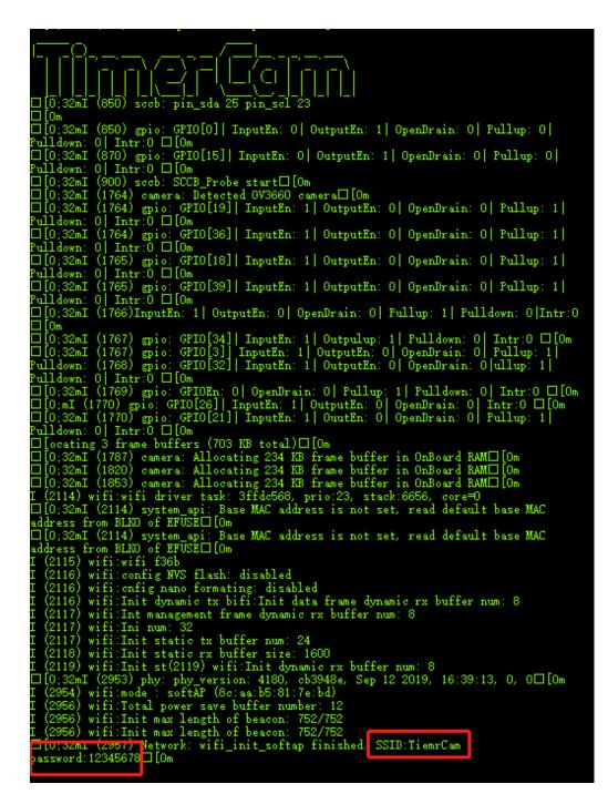
2. After waitting for a few seconds, Wi-Fi scan a AP named "TimerCam" with your computer(or mobile phone), and connect it.
