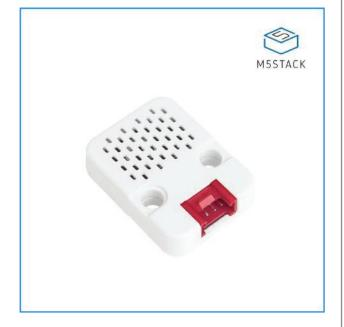
This is plugged into Port1 the I2C port. Once the CM4Stack has booted up we need to check that the I2C services have been enabled in the os. To find this out, you need to open the Raspberry Pi configuration tool found in the Preferences menu.
