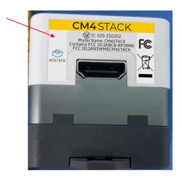
The label shown shall be permanently affixed at a conspicuous location on the device and be readily visible to the time purchase (Labeling requirements per 2.295)
