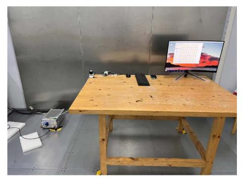
**Radiated Emissions Test View (Above 1GHz)**
