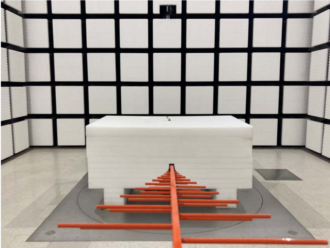
Radiated Emission Below 1GHz near View WIFI
