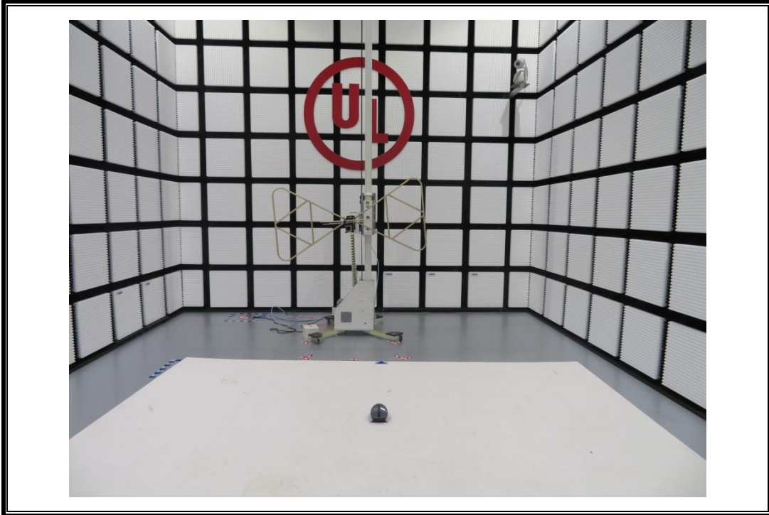
RADIATED RF MEASUREMENT SETUP (ABOVE 1 GHz- X axis)
