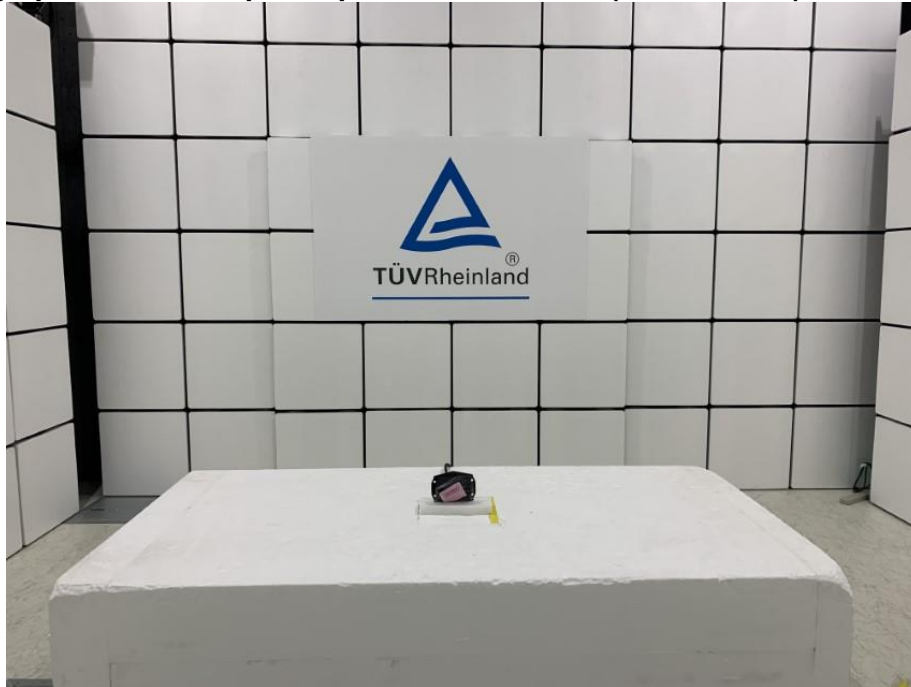
Photograph 2: Test Setup for Spurious Emissions (Front View 2)
