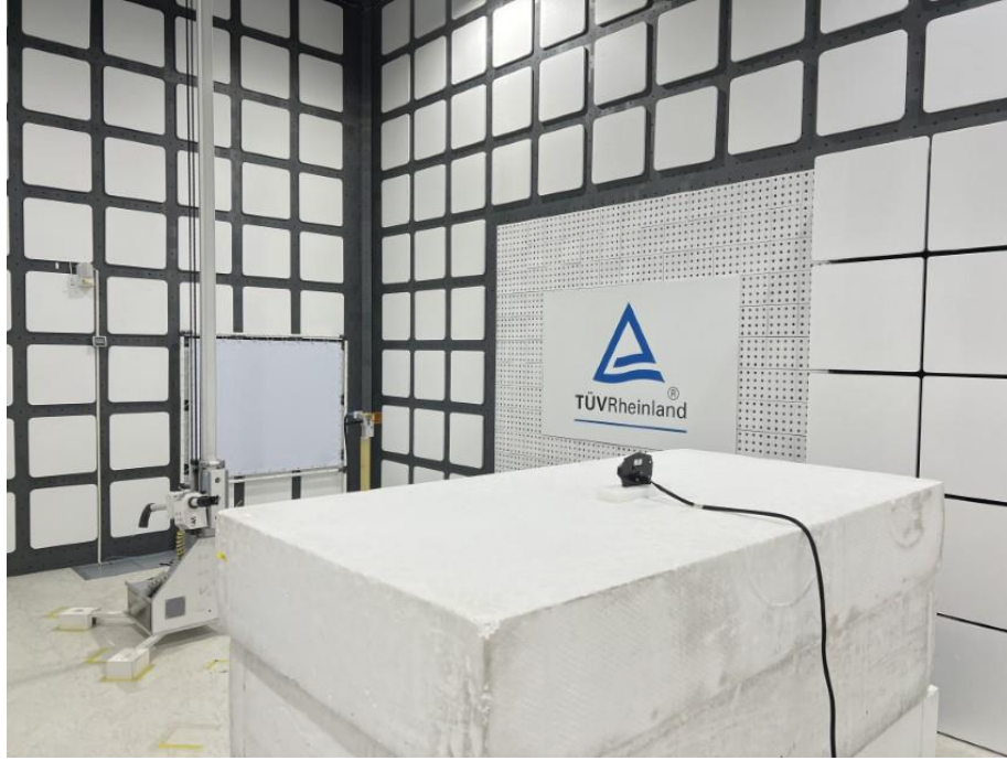
Photograph 8: Test Setup for Spurious Emissions (Back View 6)
