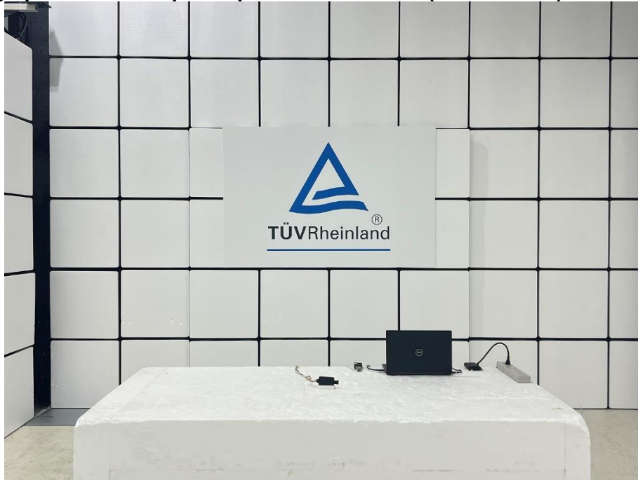
Photograph 2: Test Setup for Spurious Emissions (Front View 2)
