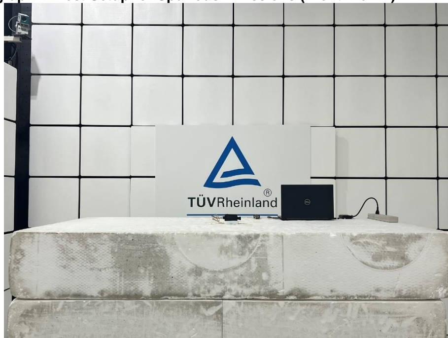
Photograph 2: Test Setup for Spurious Emissions (Front View 2)
