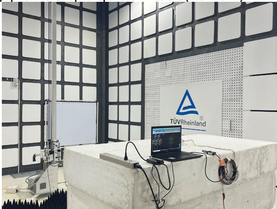
Photograph 6: Test Setup for Spurious Emissions (Back View 4)
