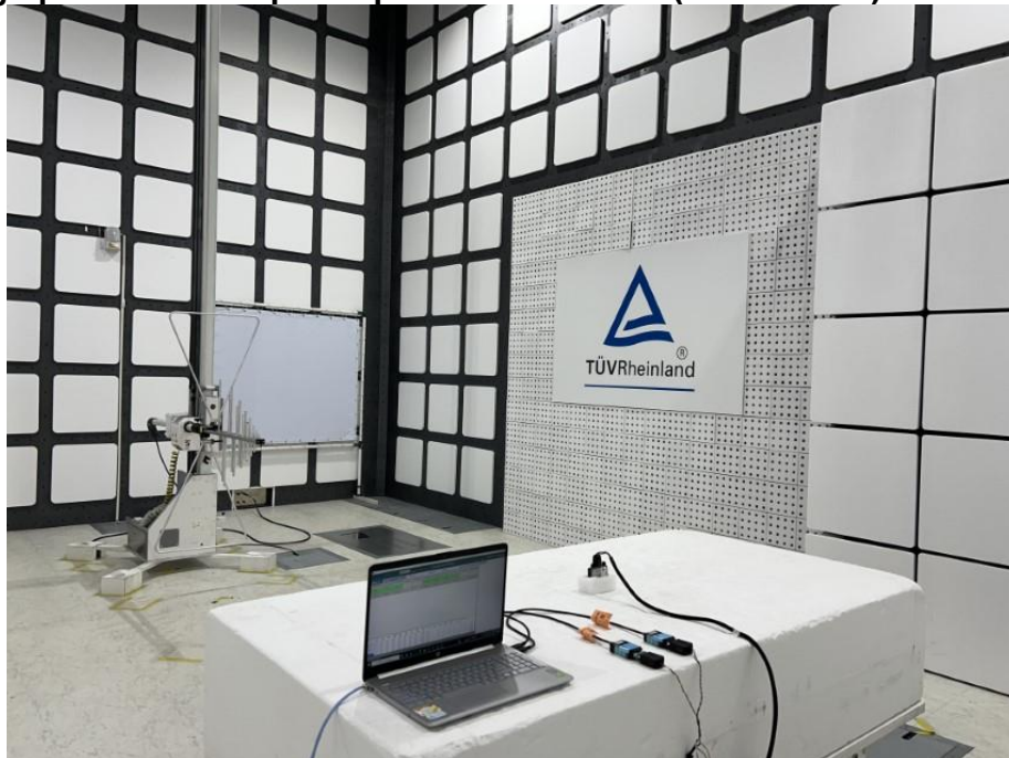
Photograph 4: Test Setup for Spurious Emissions (Back View 2)
