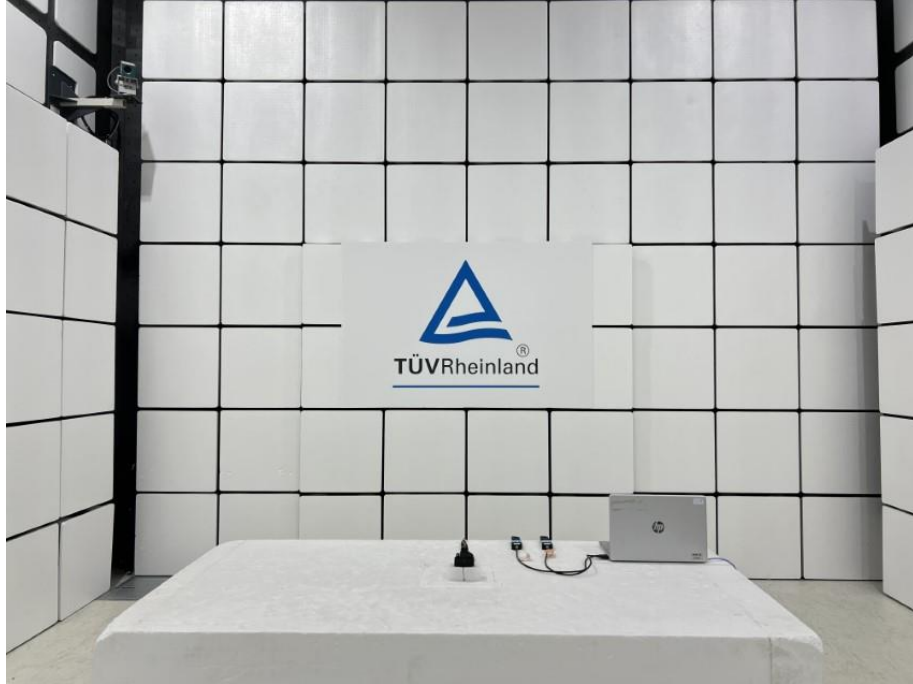
Photograph 2: Test Setup for Spurious Emissions (Front View 2)
