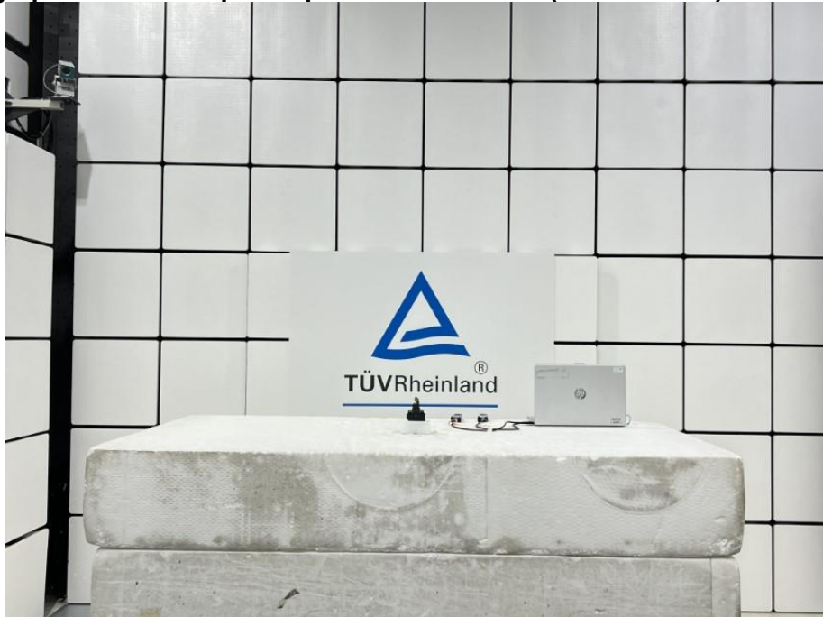
Photograph 2: Test Setup for Spurious Emissions (Front View 2)
