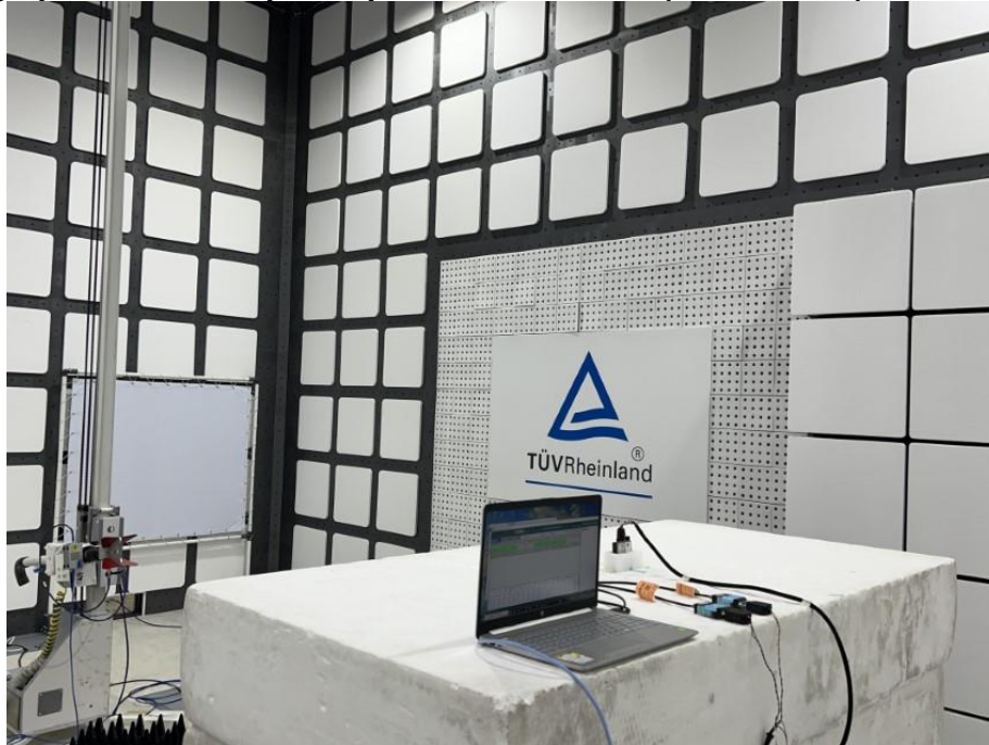
Photograph 5: Test Setup for Spurious Emissions (Back View 3)
