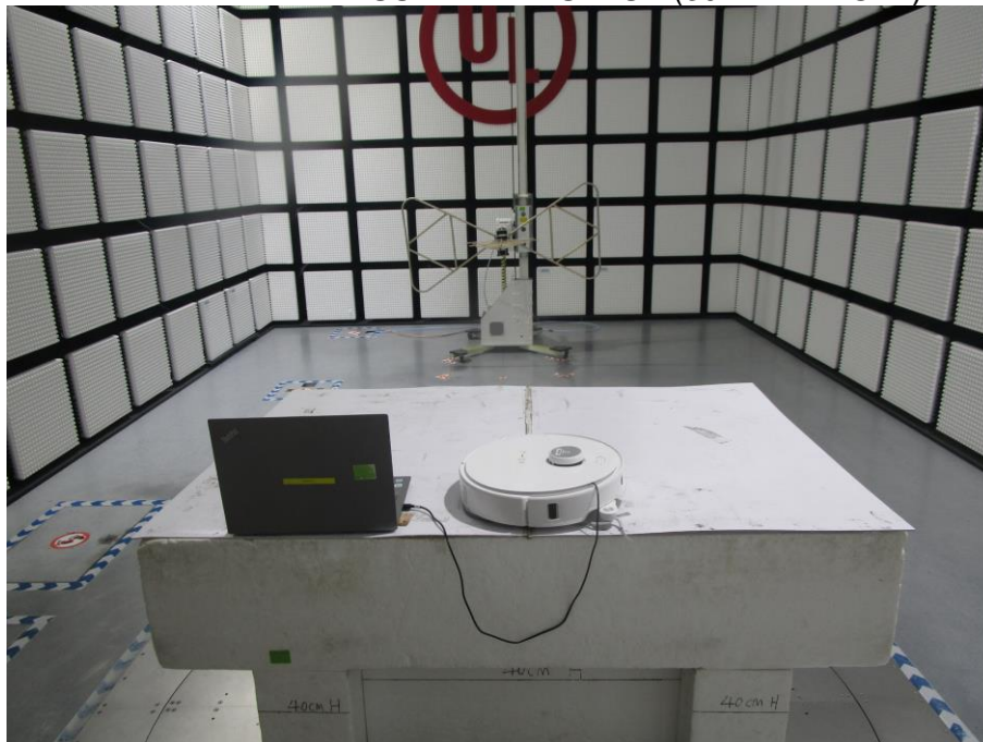
RADIATED RF MEASUREMENT SETUP (30MHz ~ 1 GHz)
