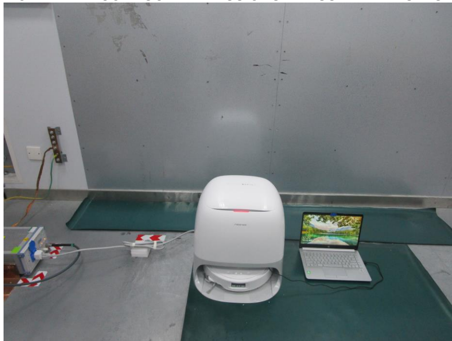
POWERLINE CONDUCTED EMISSIONS MEASUREMENT SETUP
