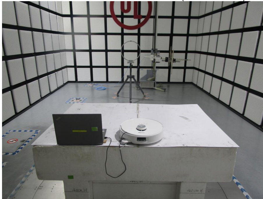
RADIATED RF MEASUREMENT SETUP (9kHz ~ 30 MHz)
