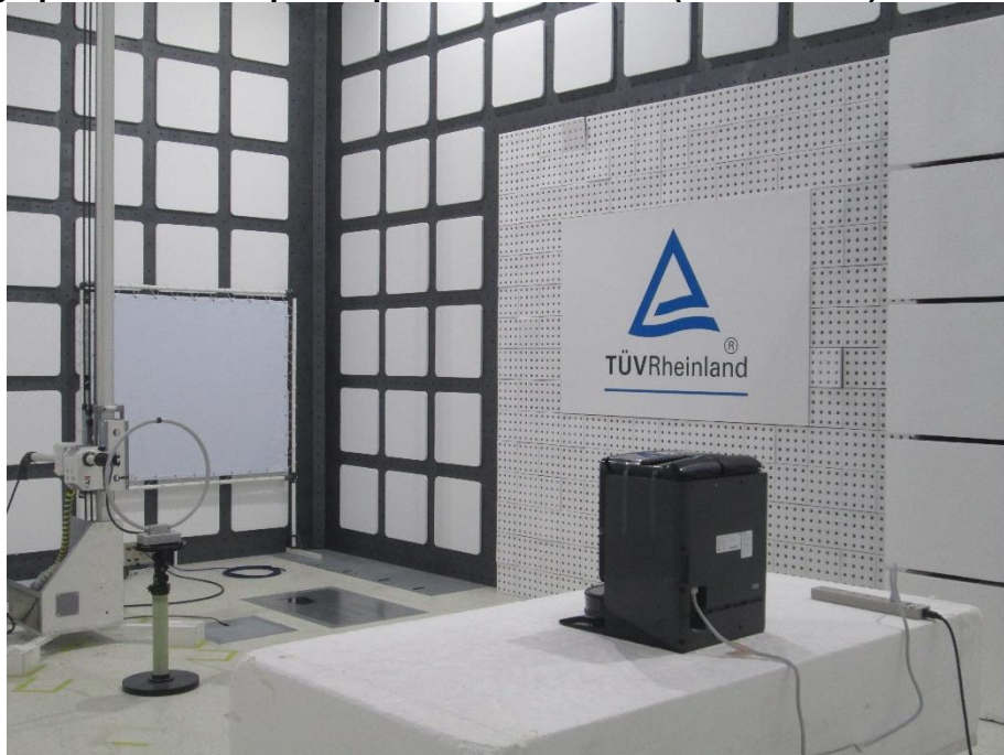
Photograph 4: Test Setup for Spurious Emissions (Back View 2)
