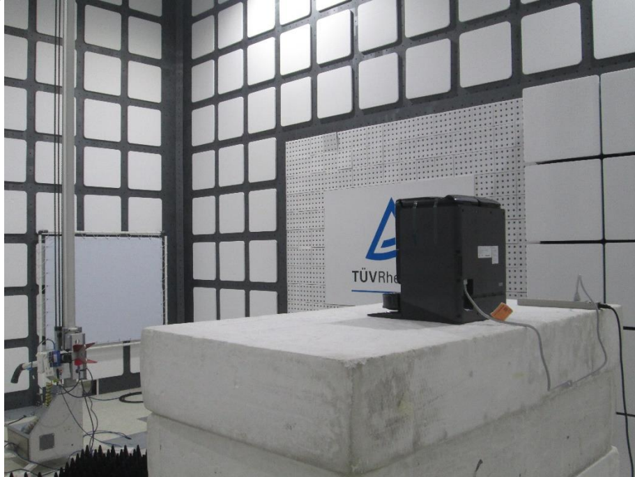
Photograph 6: Test Setup for Spurious Emissions (Back View 4)
