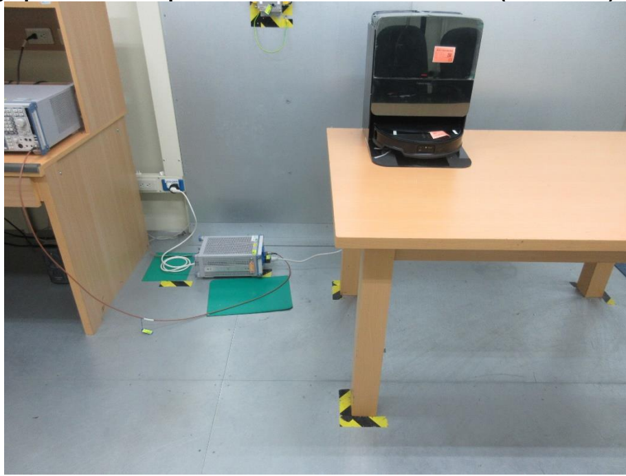
Photograph 9: Test Setup for Mains Conducted Emissions (Back View)
