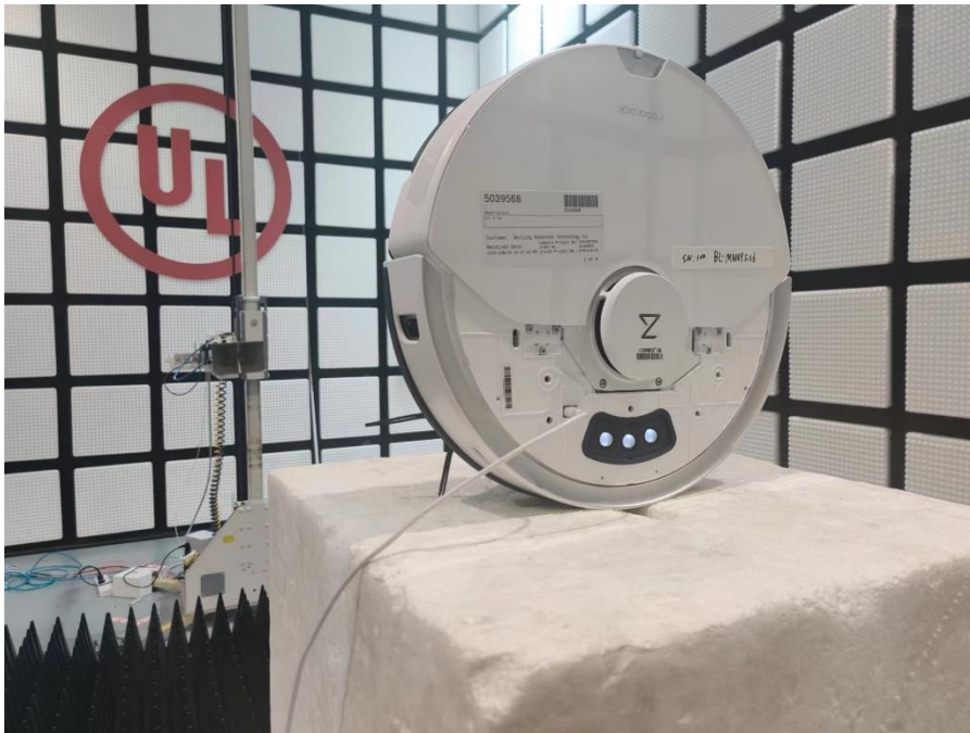
Radiated Disturbance Setup (Above 1 GHz – Y axis)
