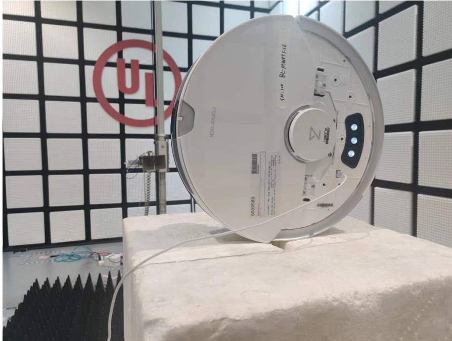
Radiated Disturbance Setup (Above 1 GHz – Z axis)
