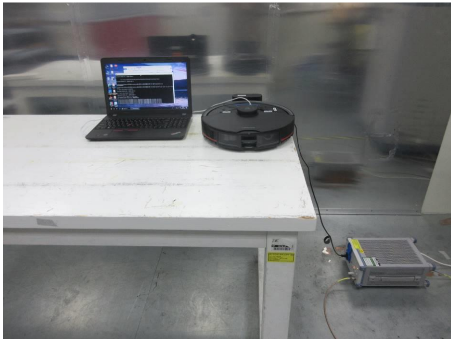
POWERLINE CONDUCTED EMISSIONS MEASUREMENT SETUP
