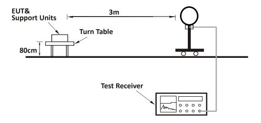
For Radiated emission 30MHz to 1GHz:
