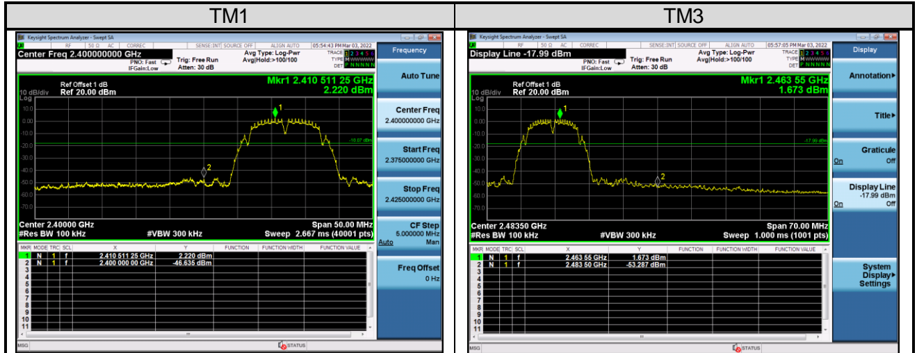
Figure 7: Conducted Band Edge
