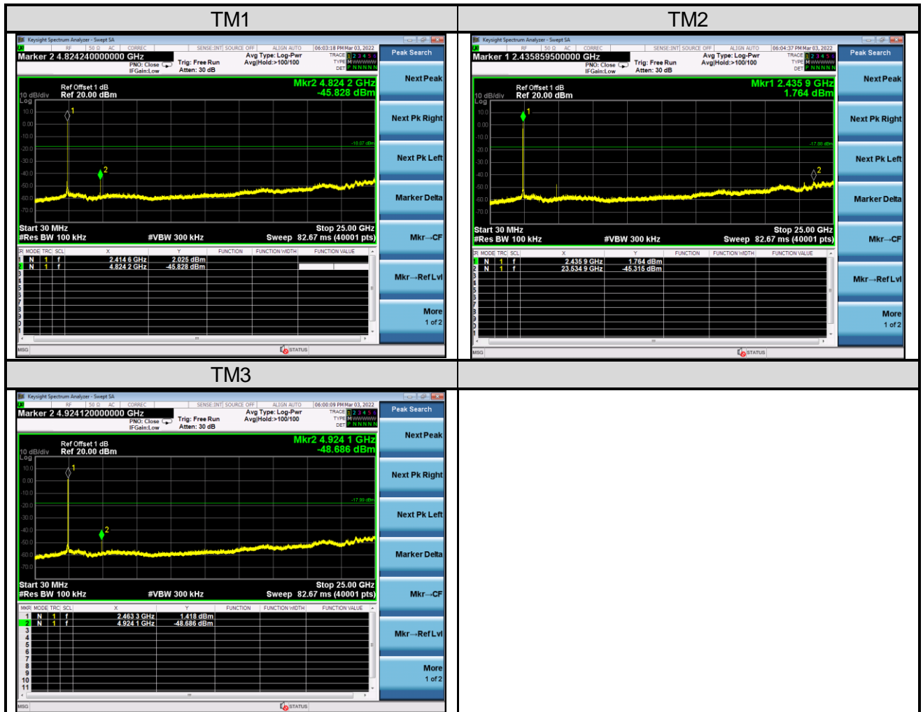
Figure 6: Conducted Spurious Emission
