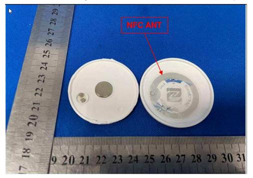
ANTENNA TYPE for NFC: Loop antenna Frequency : 13.56MHZ Gain: N/A
