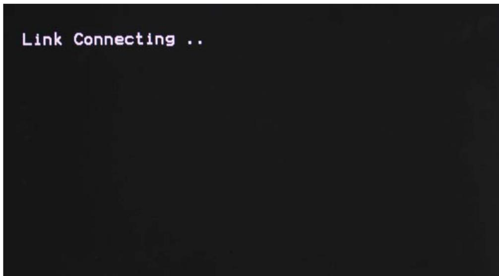
h) The system will spend 20-30 seconds on constructing communication link, and the real link period will depend on the current wireless channel condition. When wireless link is set up, 'RSSI' light will light and indicate current received wireless signal strength, as well 'video' indicators will light, and then connected HD monitor will display the video and audio accordingly.
