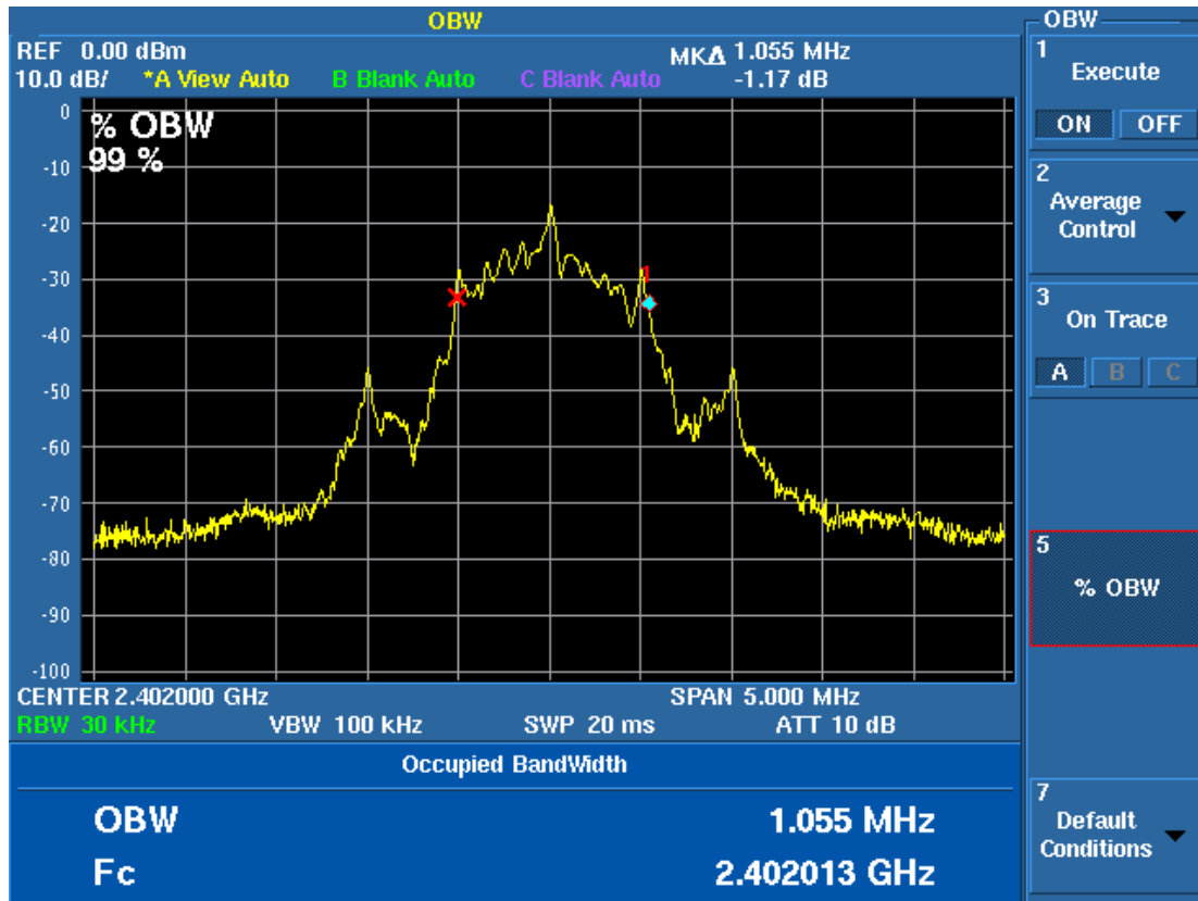
Figure 2. Occupied Bandwidth Plot
