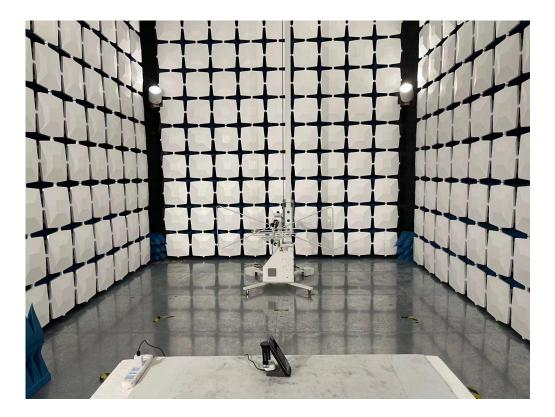
Blow 1GHz for radiated emission test setup
