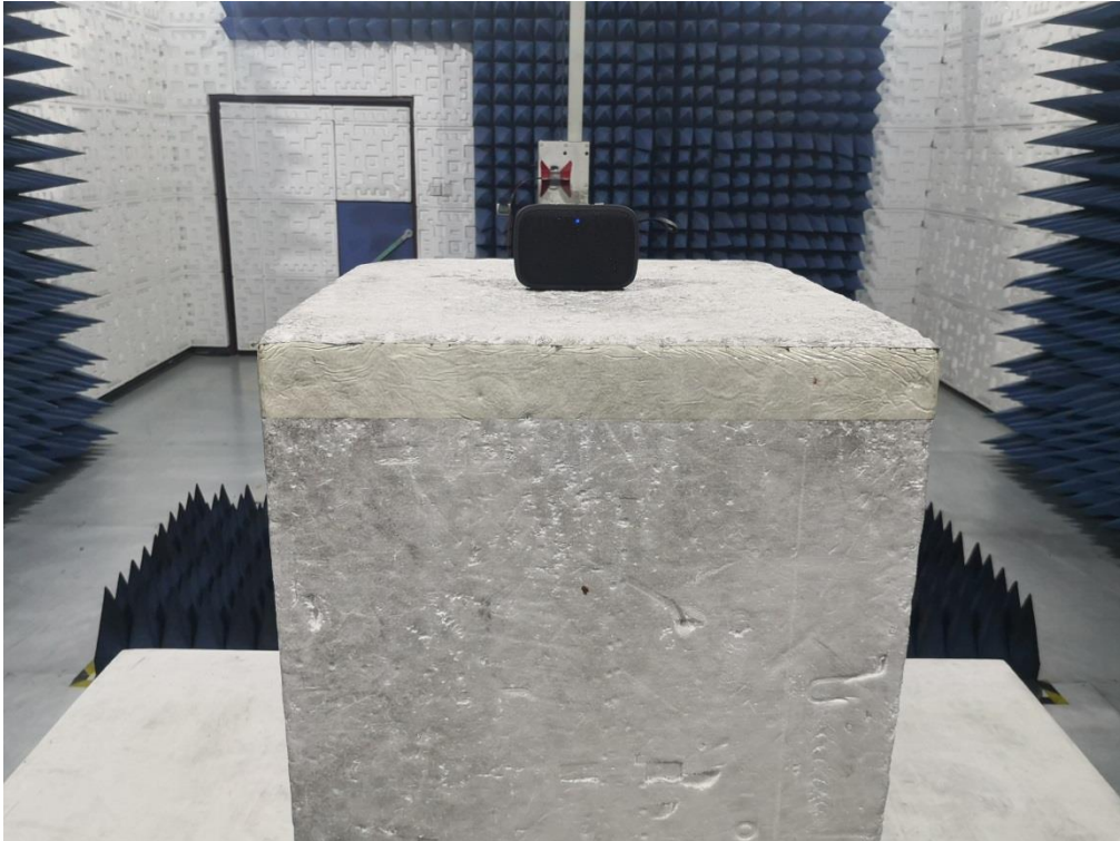
RADIATED EMISSION TEST SETUP ABOVE 1GHZ
