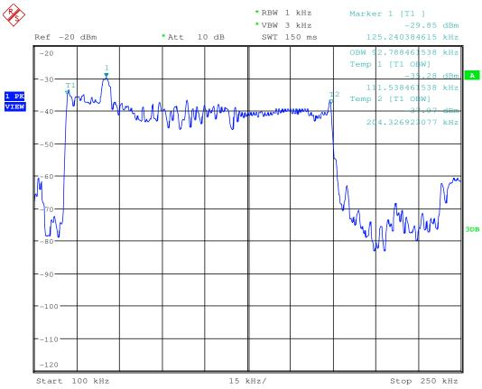
According the test data above, the fundamental wave is not fall in the restricted band 90KHz-110KHz, the field strength also meet the 15.209 requirement, test data please refer to Radiated Emissions (9kHz-30MHz), so this test is Pass.
