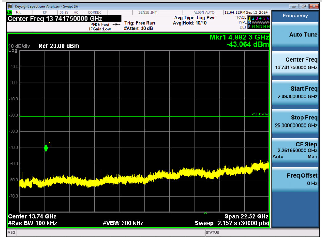
Test_Graph_BR_ANT1_2441_1Mbps_Higher Band Emissions
