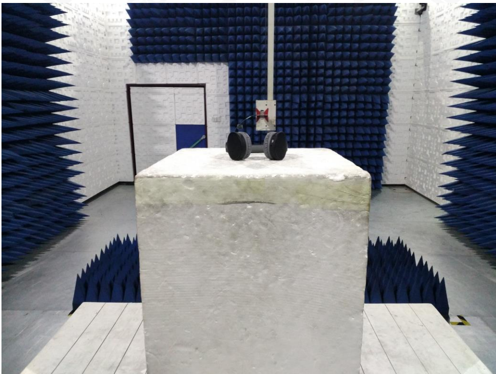
RADIATED EMISSION TEST SETUP ABOVE 1GHZ
