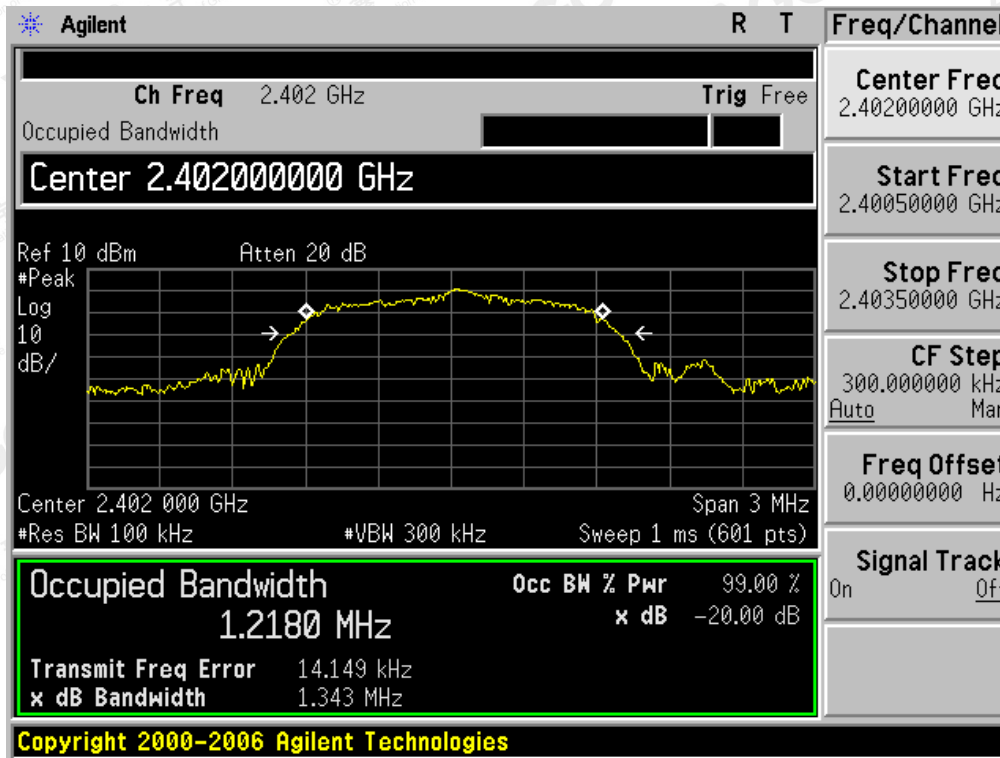
TEST PLOT OF BANDWIDTH FOR LOW CHANNEL
