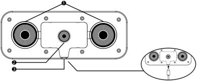
\*Connect USB-C charging cable to USB-C connection point. Connect other end of cable to a suitable power source.
