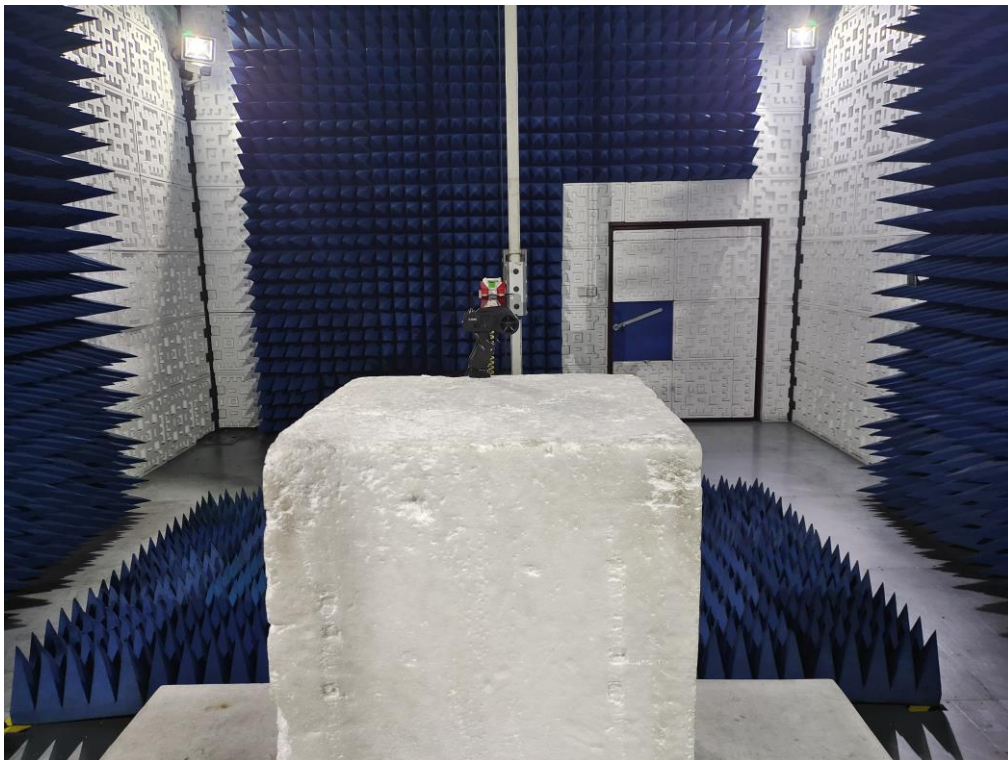
RADIATED EMISSION TEST SETUP ABOVE 1GHz
