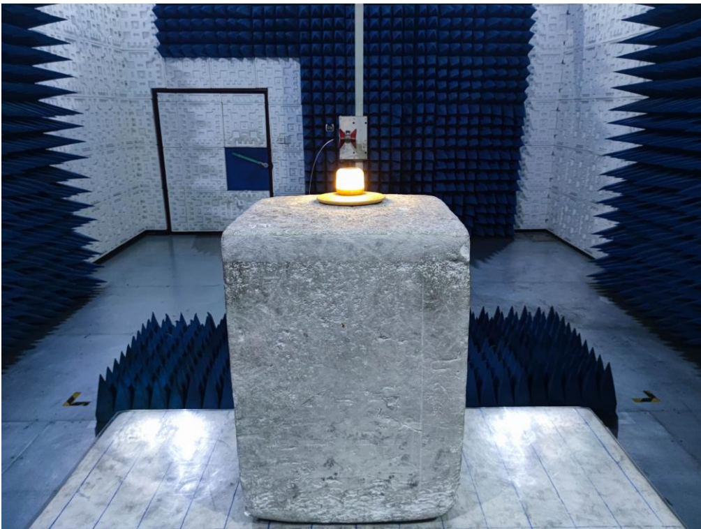
RADIATED EMISSION TEST SETUP ABOVE 1GHz
