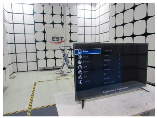
Radiated Test (1000-25000 MHz)
