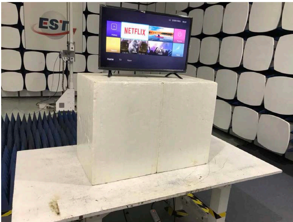
Radiated Test(Above 1 GHz)
