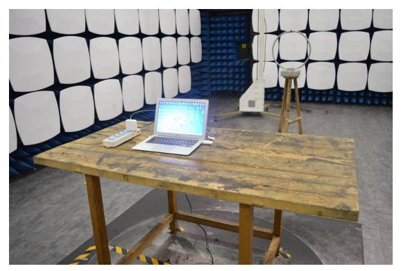
3. Radiated emission (9KHz-30MHz)
