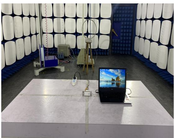
3. Radiated emission (9KHz-30MHz)
