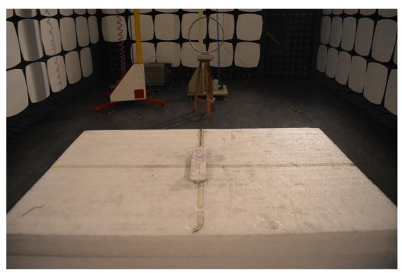
3. Radiated emission (9KHz-30MHz)
