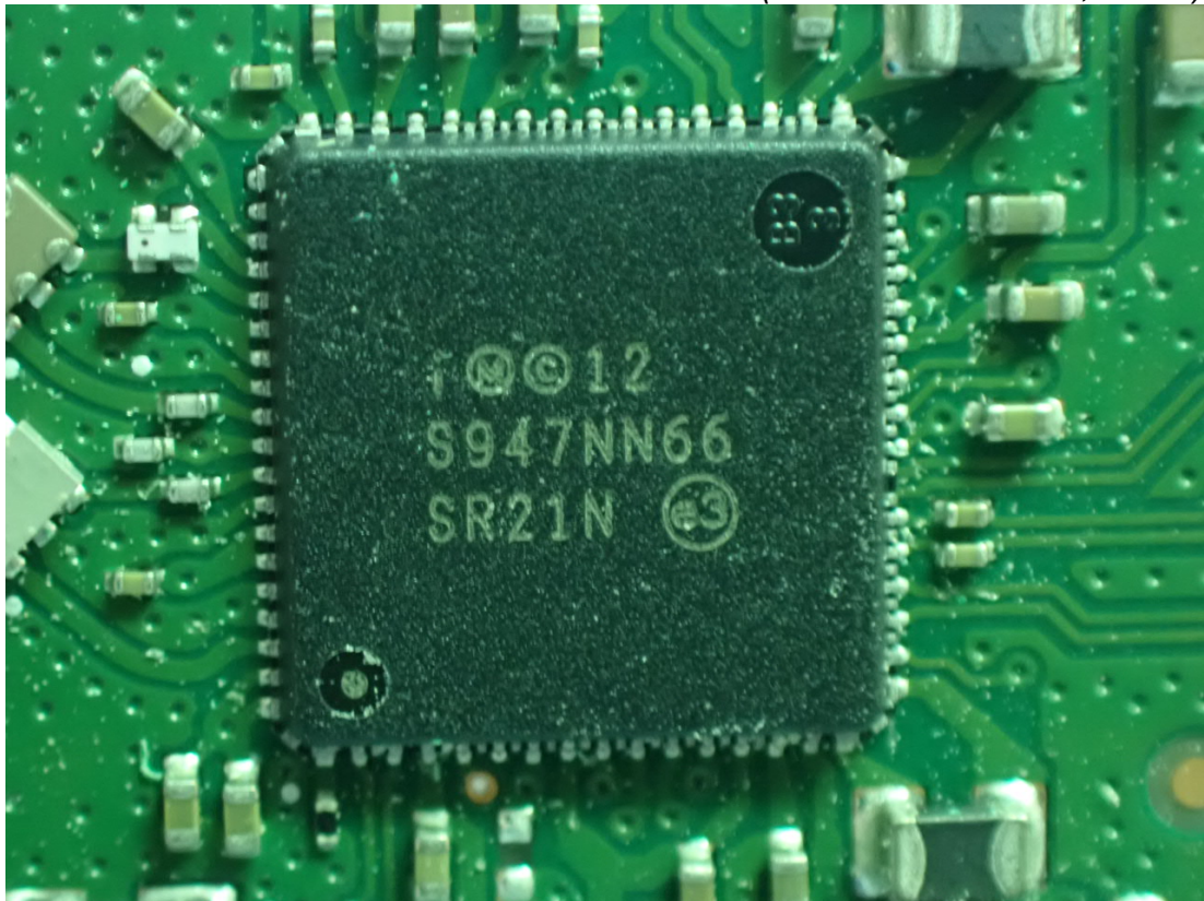
Figure 31 Internal View (WLAN Combo Card, RF IC)
