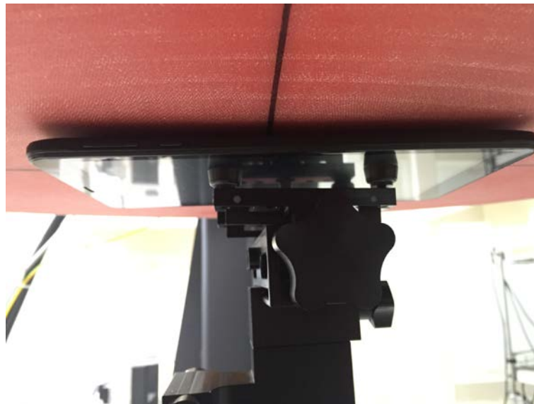
Test Position 1 - Body-worn, the rear side of the EUT towards phantom (The distance was 0mm)
